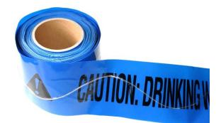
Wenac Warning Tape is made of tough PE material with stainless steel 316 wire embedded. It is typically buried above the underground non-metal pipelines, which can be detected via a metal detector from the surface. It has been widely used to prevent from unintentional damage during excavation or digging.
